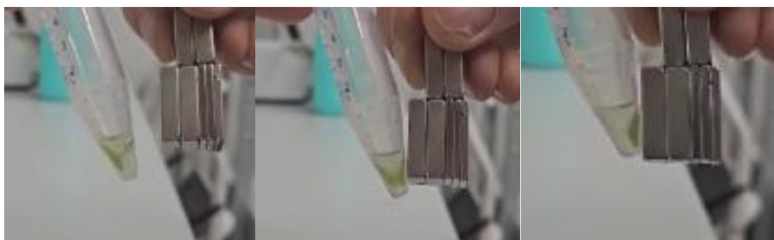
Figure 2- Microalgae coupled with PAC, PAM and the magnetic particles. In this figure is possible to visualize the microalgae following the magnetic field.
