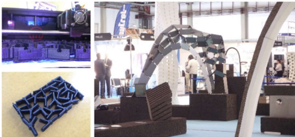
“TriArch” project - fabrication, nodes, and final structure.
