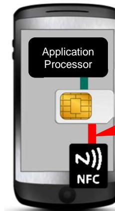
SIM-NFC connection through a single, wired interface
